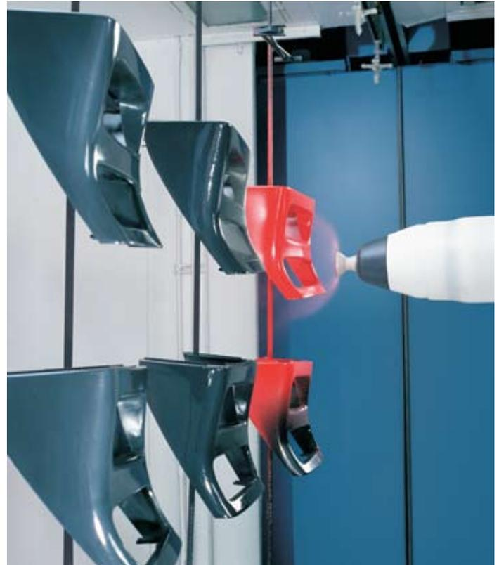
vector air for superior pattern shaping, long-life air-bearing turbine design, innovative electrostatic charging system and a proprietary composite cup.
